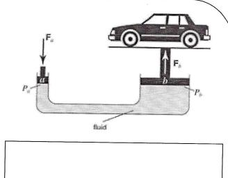
Example: Suppose that the area of the small piston is  $50 \text{cm}^2$  and it is pushed with a force of 50 N. How much force is exerted upward by the large piston with an area of  $2.0 \text{ m}^2$ ?
